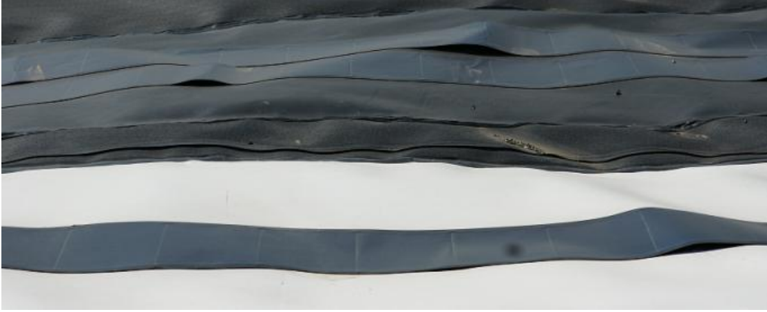
Figure 5. Various types of (HD)PE liners with laminated PV-module (6m length)
