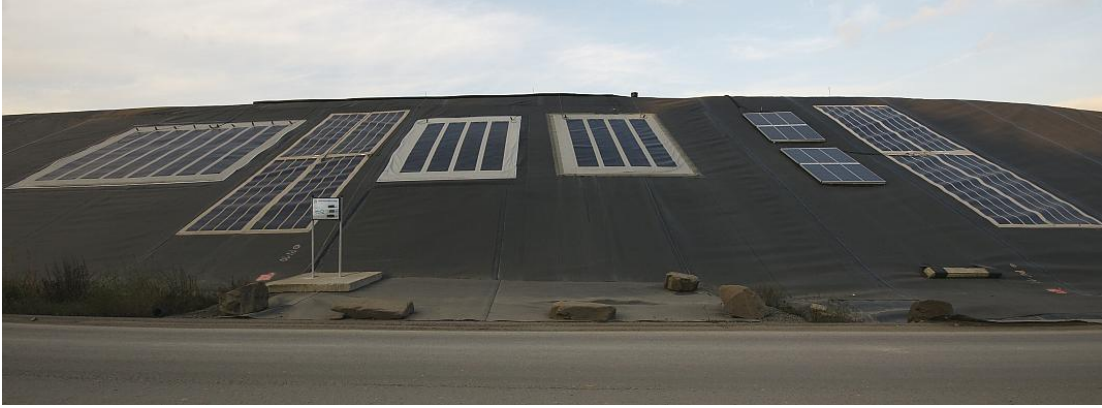
Figure 2. Various roof membrane composites on HD-PE landfill cover and crystalline reference fields (second from right side) on the steep slope
