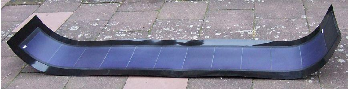
Figure 4. Early prototype of HD-PE liner with laminated PV-module (3m length)
